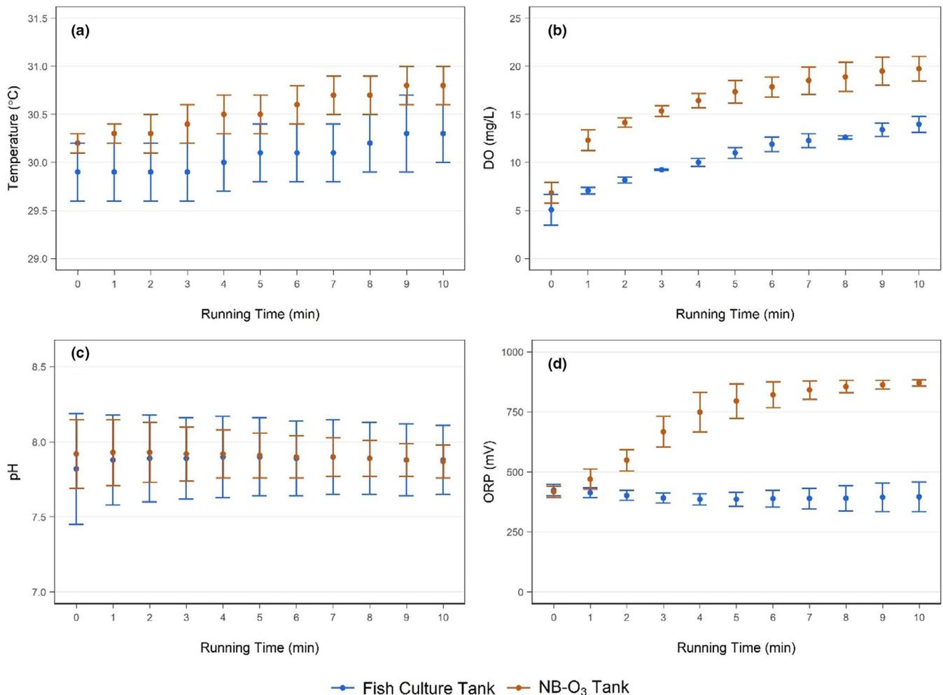
**FIGURE 2** Measurement of water parameters including temperature (a), DO (b), pH (c), and ORP (d) during 10-min NB-O<sub>3</sub> treatment with 2 L/min oxygen input in MRS. Value of water parameters is mean  $\pm$  SD ( $n = 3$ )
